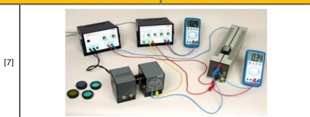
**Photoelectric /Determining Plank constant**
